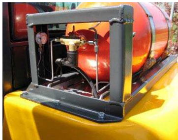
Natural gas storage facility with SOL union
